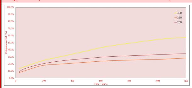
Note: The compression set at 200°C is slightly higher than 250°C because the higher temperature aids its recovery. Over longer time periods it is expected that the 200°C compression set will outlast the 250°C compression set.
